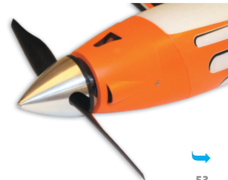
The new aluminum spinner was changed in the course of product care against the one made of plastic.
